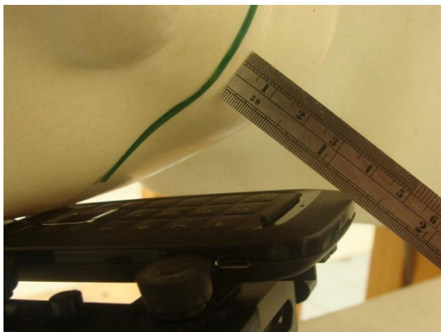
Right Cheek position - Separation distance 4cm between mouth and antenna
