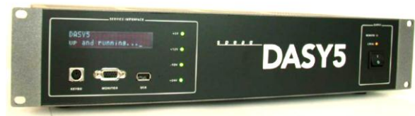
Fig. 5.9 Photo of Server for DASY5
