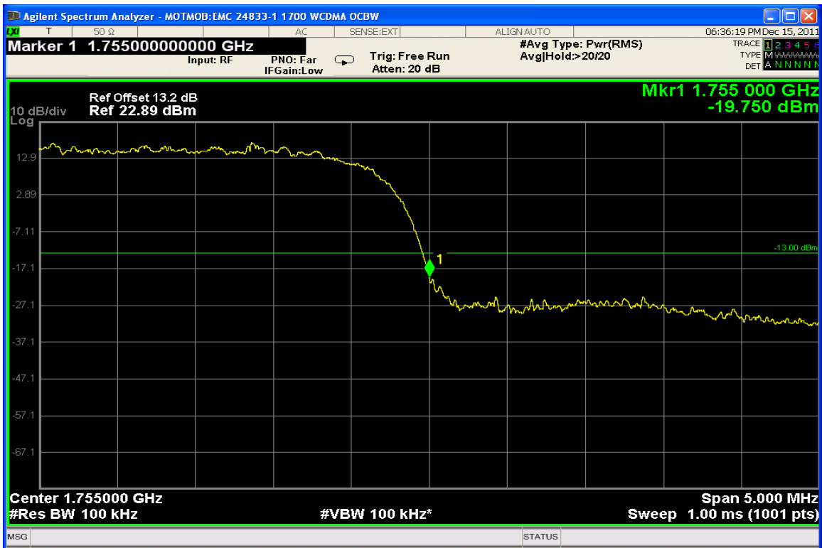
WCDMA 1700 – Upper Band Edge – Channel 1513 (1752.6 MHz)
