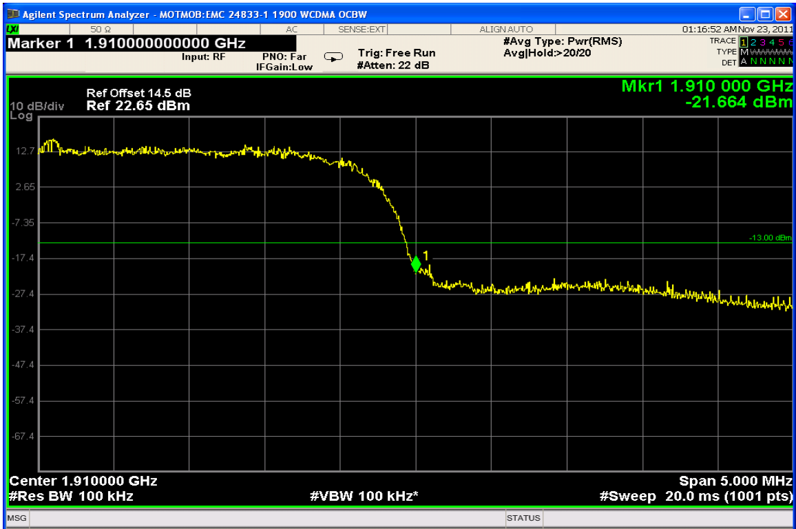
WCDMA 1900 – Upper Band Edge – Channel 9538 (1907.60 MHz)
