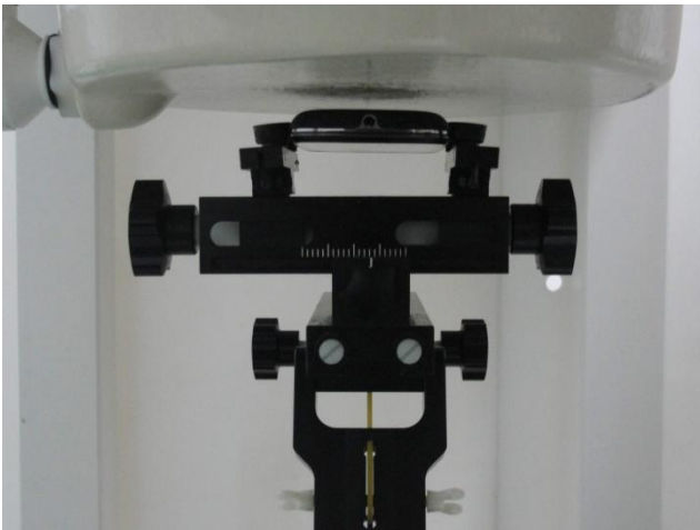
Rear Face of the DUT with Phantom 1 cm Gap (EUT without Earphone)
