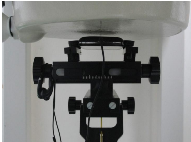
Rear Face of the DUT with Phantom 1 cm Gap (EUT with Earphone)
