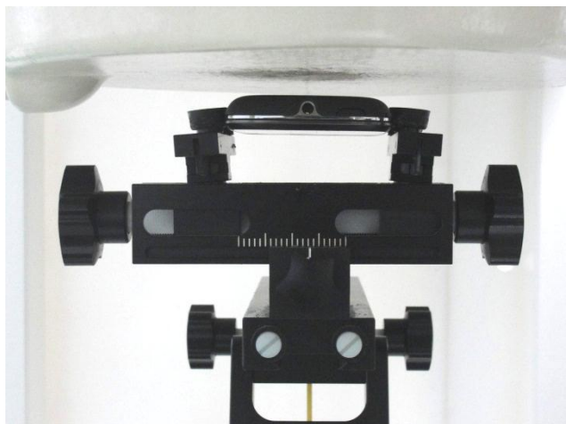
Rear Face of the DUT 1 cm Gap
