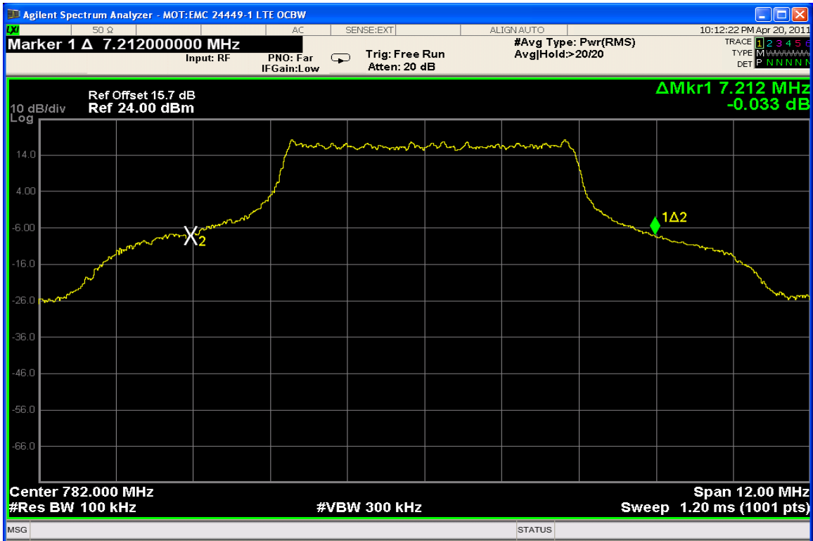
LTE – Band 13 - 16 QAM, Start RB: 13, RB Allocation 50%
