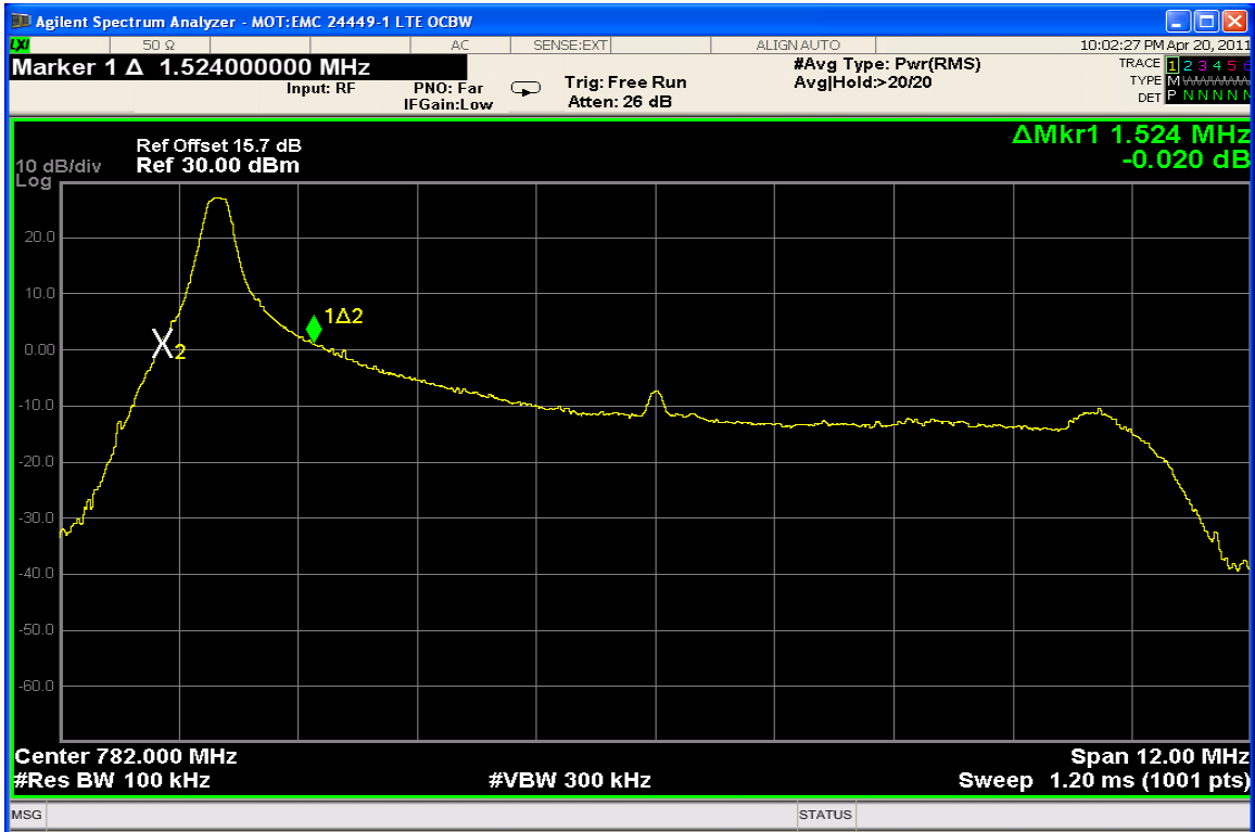
LTE – Band 13 - 16 QAM, Start RB: 0, 1RB@ low end
