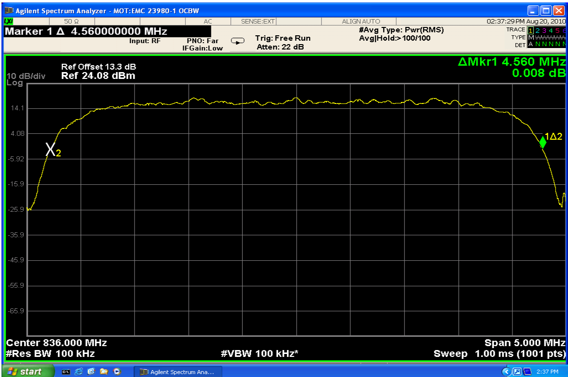
WCDMA 850 – Occupied Bandwidth – Channel 4180 (836.00 MHz)
