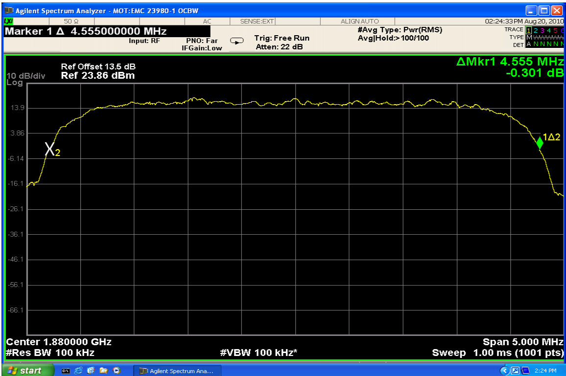
WCDMA 1900 – Occupied Bandwidth – Channel 9400 (1880.00 MHz)
