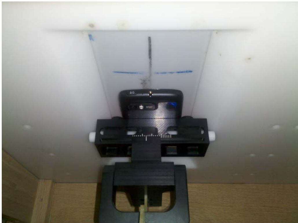
Figure 8: Mobile Hotspot Position, Front of Phone facing Phantom (10 mm separation)
