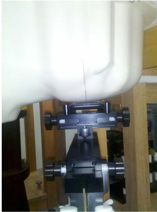
Figure 3: Cheek Position, Front of Head of Phantom
