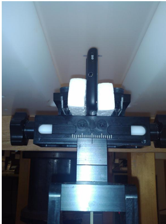
Figure 9: Mobile Hotspot Position, Right Edge of Phone facing Phantom (10 mm separation)
