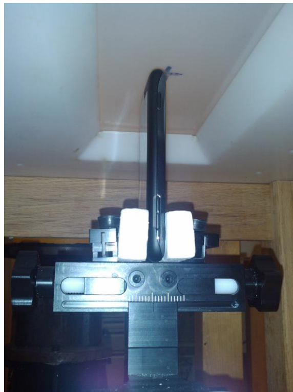
Figure 10: Mobile Hotspot Position, Bottom Edge of Phone facing Phantom (10 mm separation)
