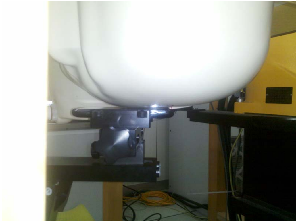
Figure 4: Cheek Position, Top of Head of Phantom
