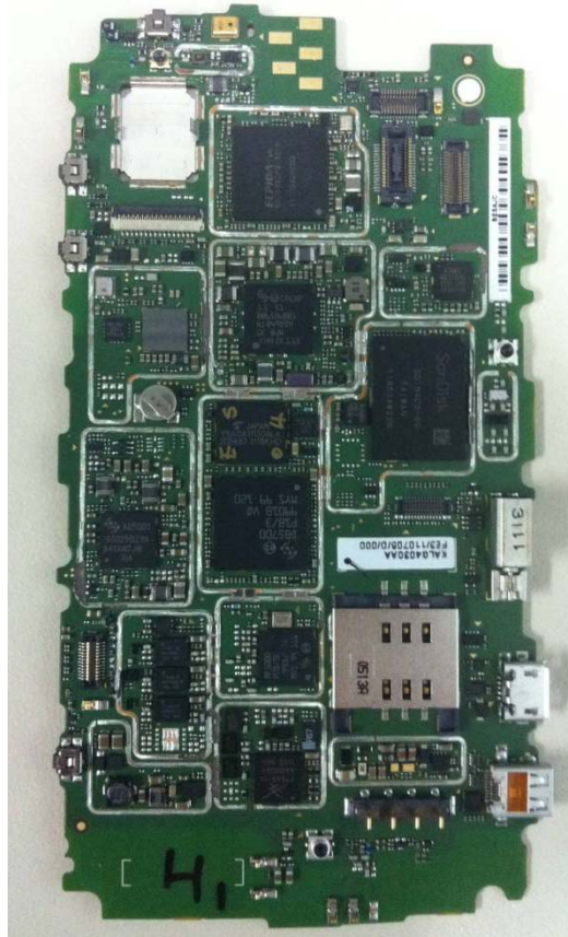
BACK OF MAIN PCB WITHOUT SHIELD CAN
