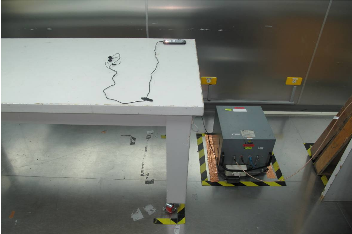
Conducted Emission Set up Photo (config 3)
