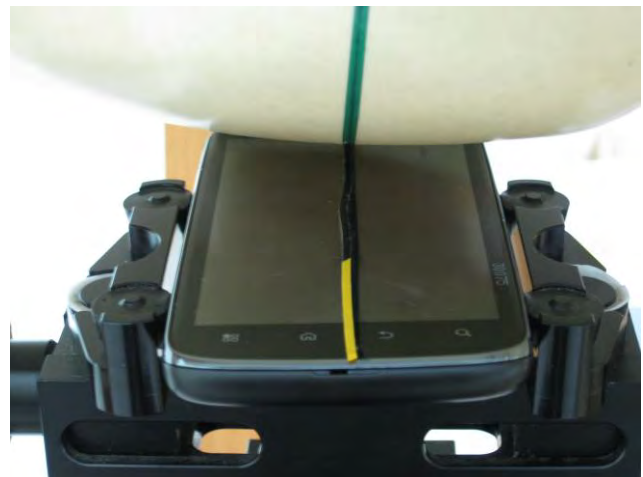
Fig.4 Right Head Section / Ear-Tilt Position(15°)
