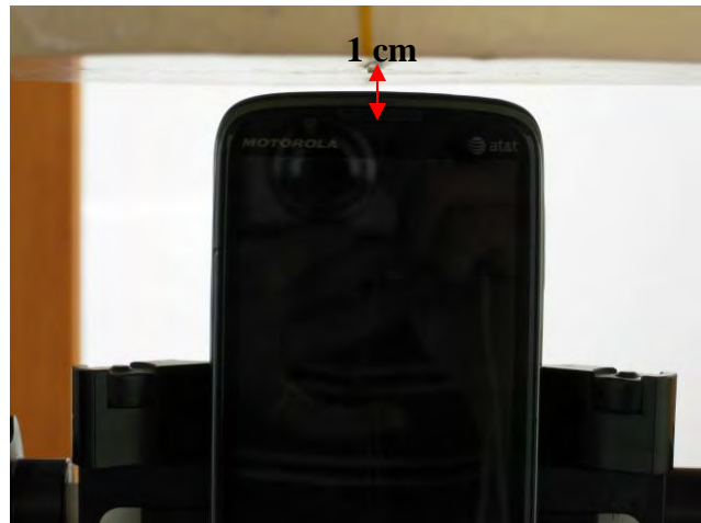
Fig.9 Hotsopt mode- EUT Top to flat phantom and distance between flat phantom and mobile phone is 1 cm.
