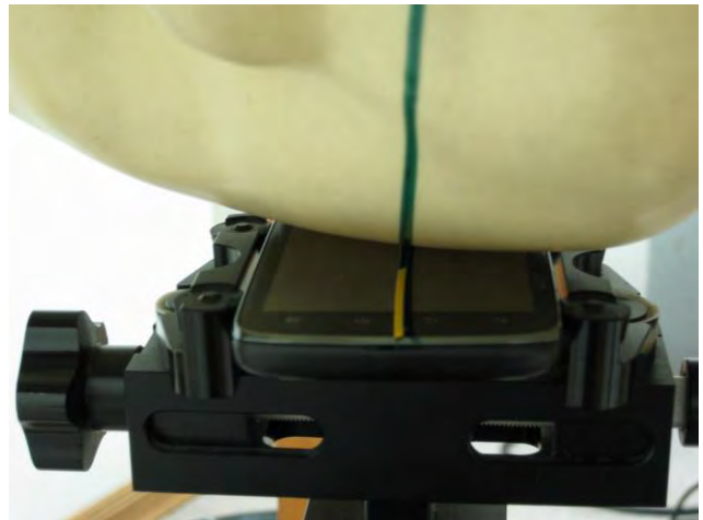
Fig.3 Right Head Section / Cheek-Touch Position
