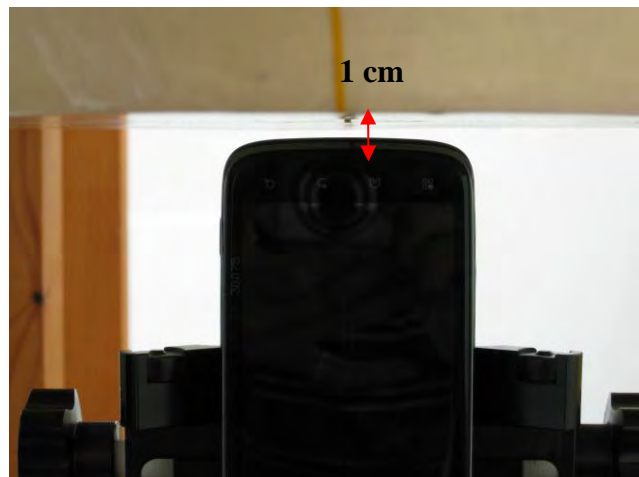
Fig.10 Hotsopt mode- EUT Bottom to flat phantom and distance between flat phantom and mobile phone is 1 cm.
