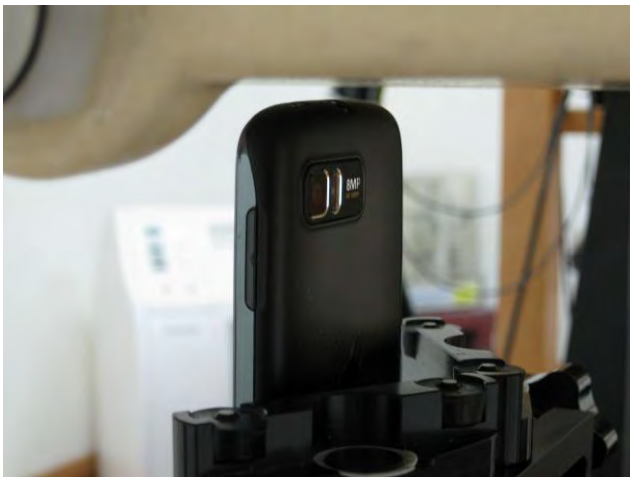
Fig.9 Hotsopt mode- EUT Top to flat phantom and distance between flat phantom and mobile phone is 1 cm.
