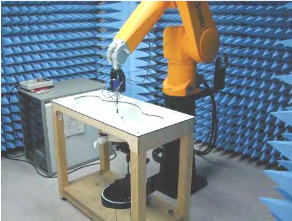
Fig.1 Photograph of the SAR measurement System
