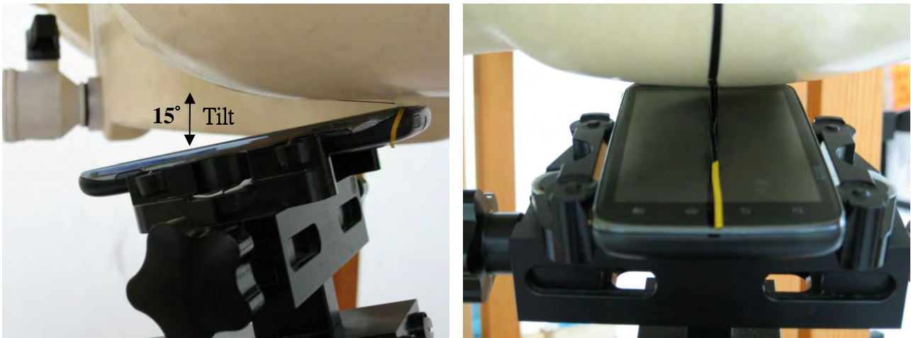
Fig.6 Left Head Section / Ear-Tilt Position(15°)
