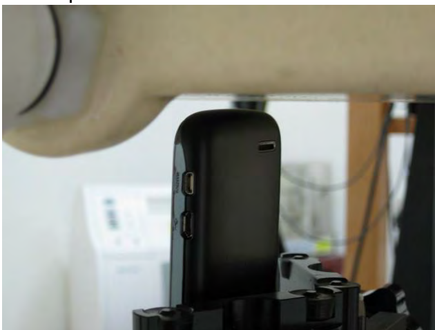
Fig.10 Hotsopt mode- EUT Bottom to flat phantom and distance between flat phantom and mobile phone is 1 cm.
