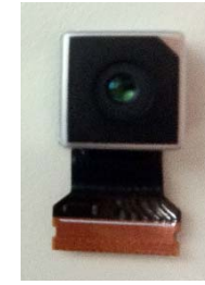
FRONT OF ASSY 8M CAMERA MODULE
