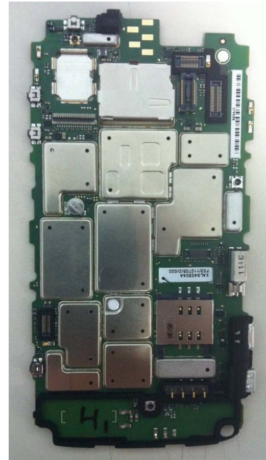
BACK OF MAIN PCB WITH RUBBERS
