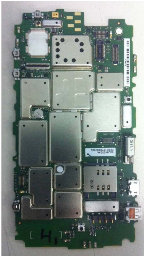
BACK OF MAIN PCB WITH SHIELD CAN
