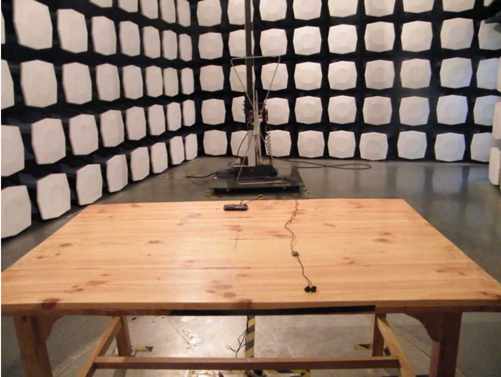
Picture 1: Radiated Emission Test Setup
