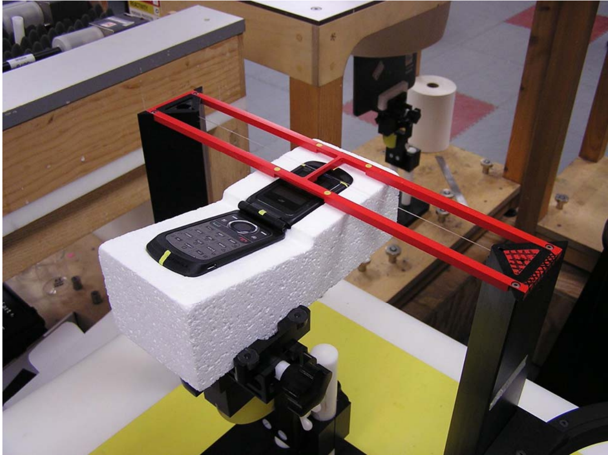
Figure 3. Positioning and Measurement for RF Emissions
