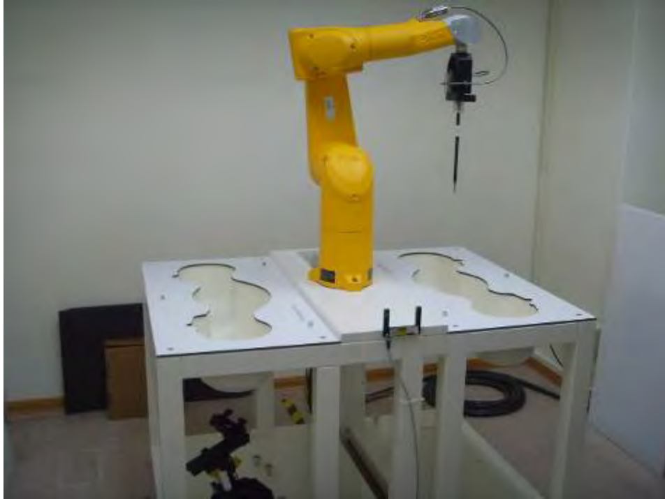
Fig.1 Photograph of the SAR measurement System
