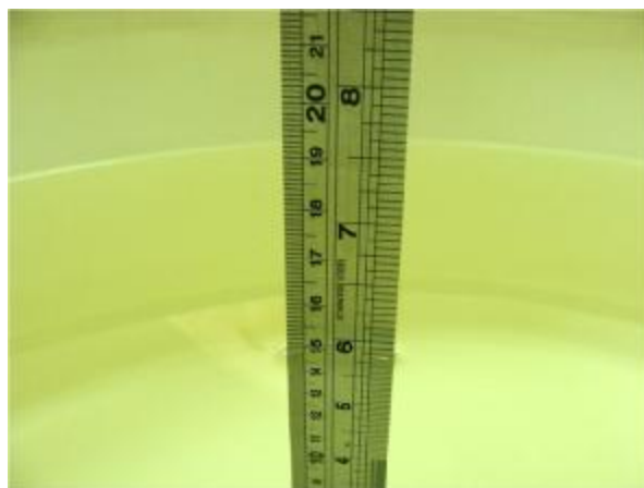
Fig 6.2 Photo of Liquid Height for Body SAR
