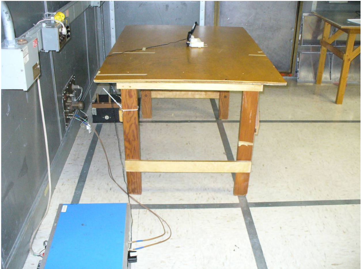
Figure 4: Conducted Emissions – Side View
