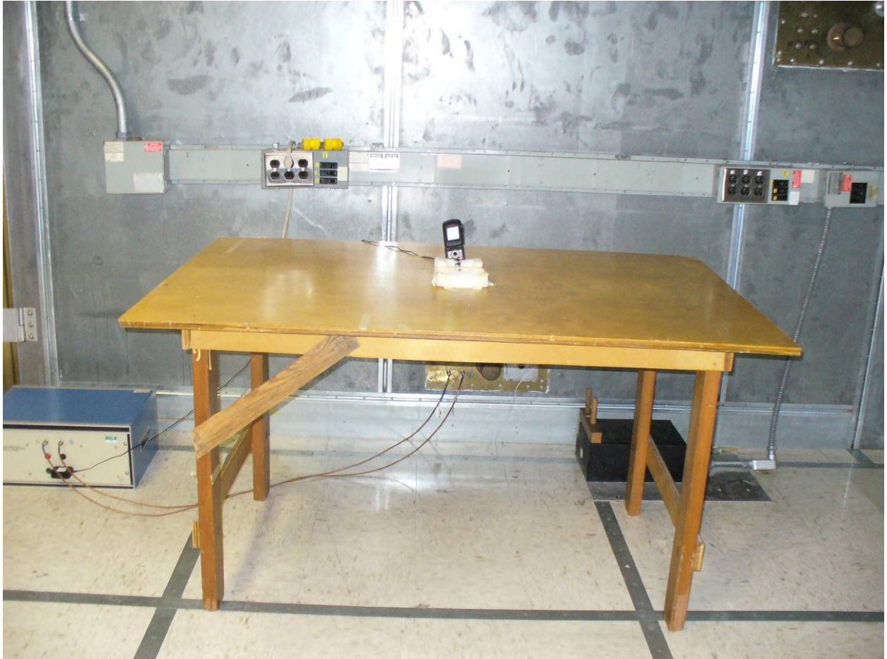
Figure 3: Conducted Emissions – Front View
