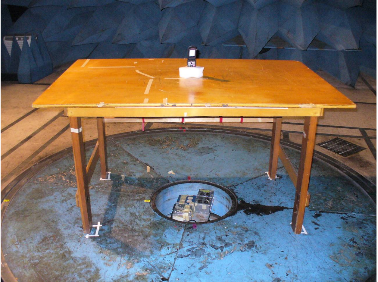
Figure 1: Radiated Emissions – Front View
