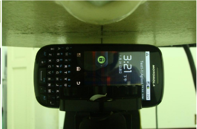
Left Side of the DUT with Phantom 1 cm Gap (DUT without Earphone)
