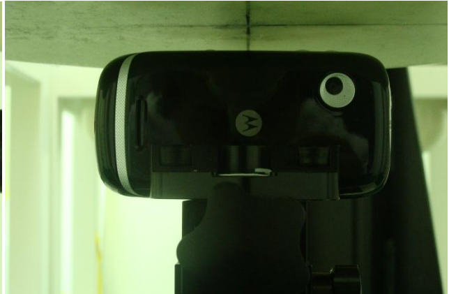
Right Side of the DUT with Phantom 1 cm Gap (DUT without Earphone)
