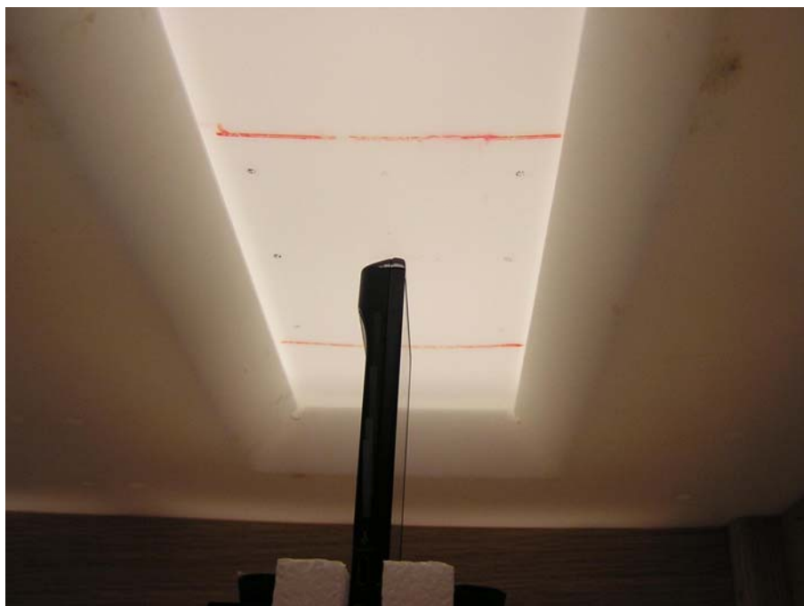
Figure 8: Mobile Hotspot Position at 10mm away from phantom Short edge of phone (top or bottom)
