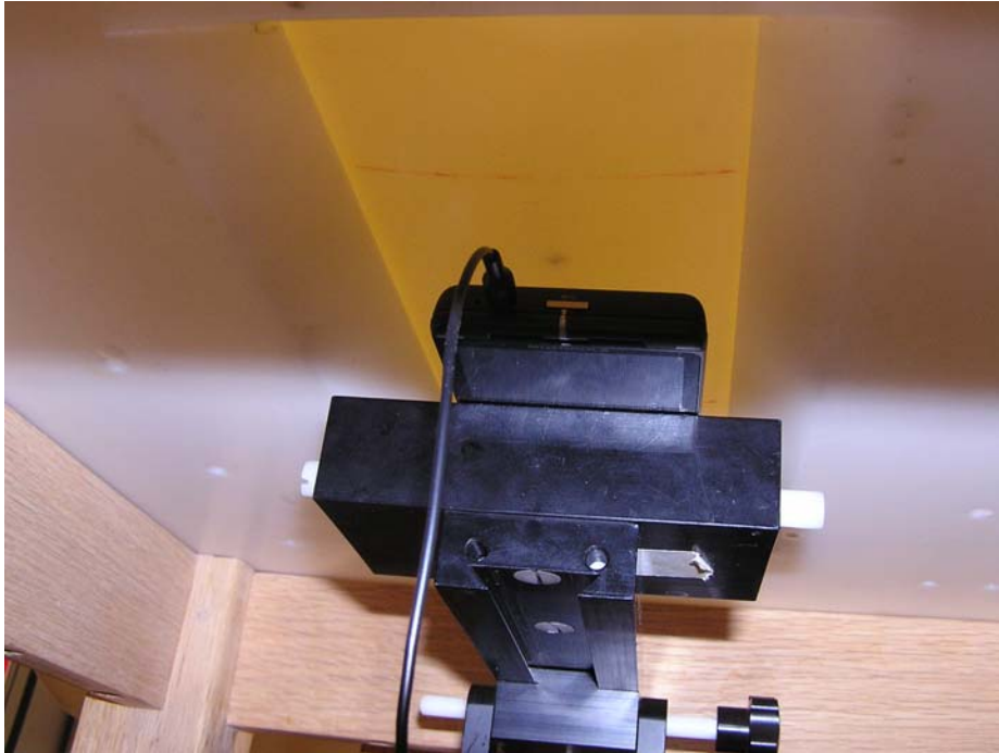
Figure 5: Body Position at 25mm away from phantom (back of phone)
