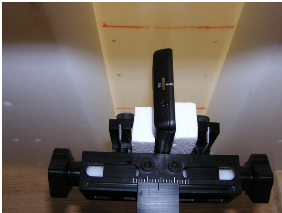
Figure 7: Mobile Hotspot Position at 10mm away from phantom Long edge of phone (right or left)
