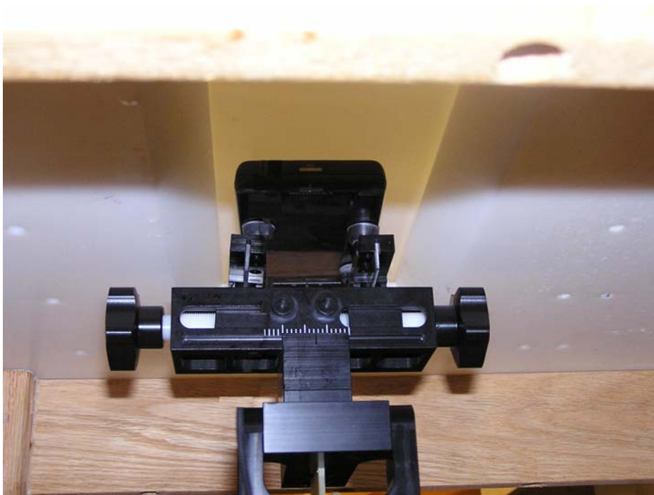
Figure 6: Mobile Hotspot Position at 10mm away from phantom (back of phone)
