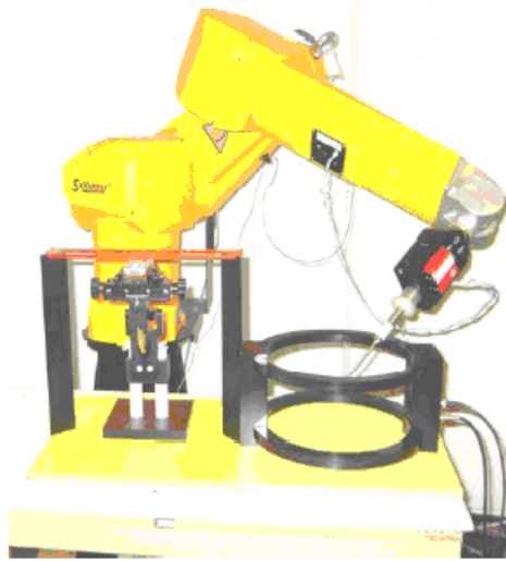
Figure 1: T-coil setup and cabling (pictures from DASY manual)
