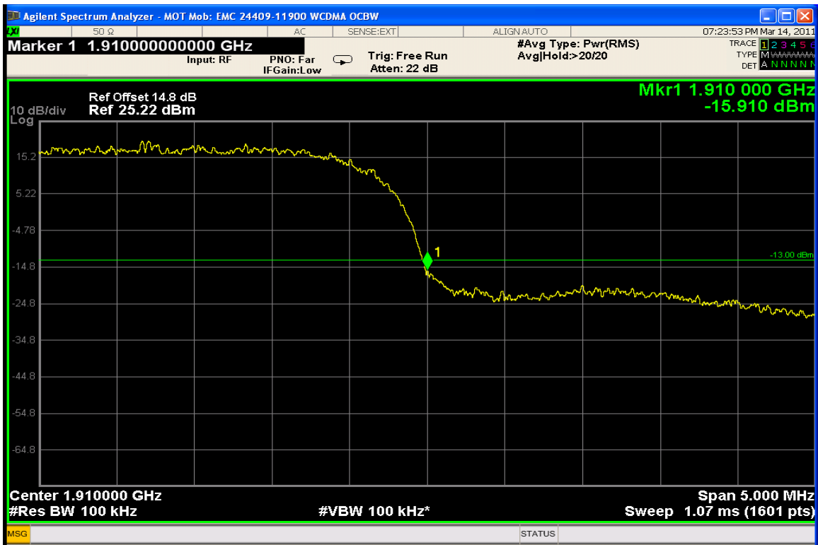
WCDMA 1900 – Upper Band Edge – Channel 9538 (1907.60 MHz)
