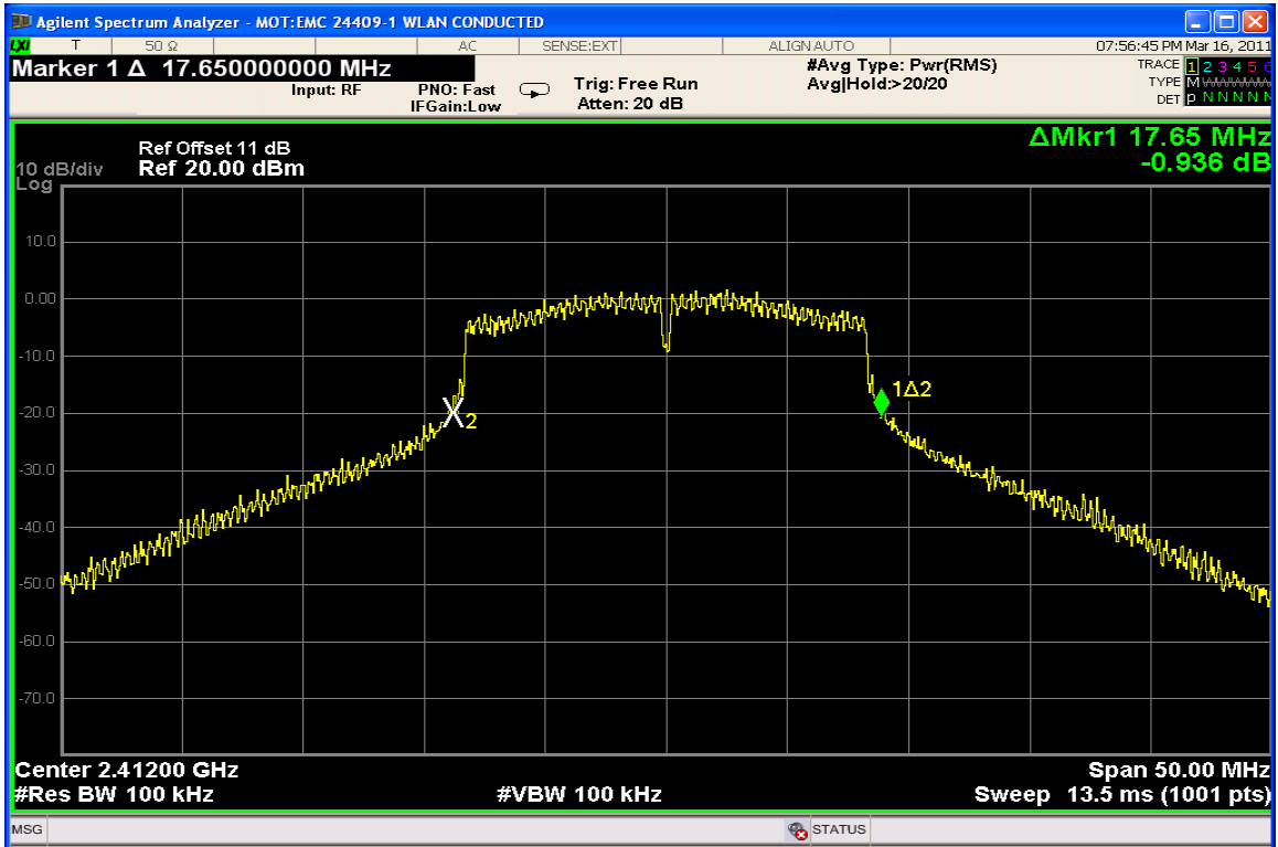
20 dB Bandwidth Channel 1 @ 9Mbps
