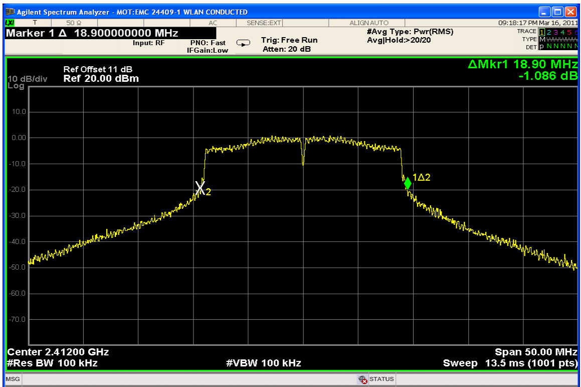
20dB Bandwidth Channel 1 @ 14.4Mbps
