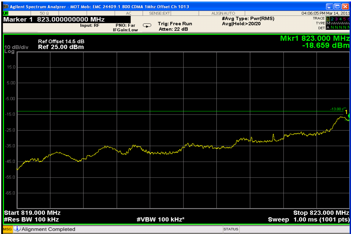
Channel 1 @ 11Mbps – Lower Band Edge
