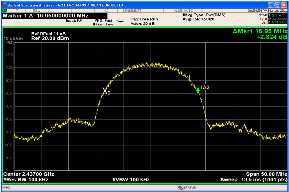
20 dB Bandwidth Channel 6 @ 11Mbps
