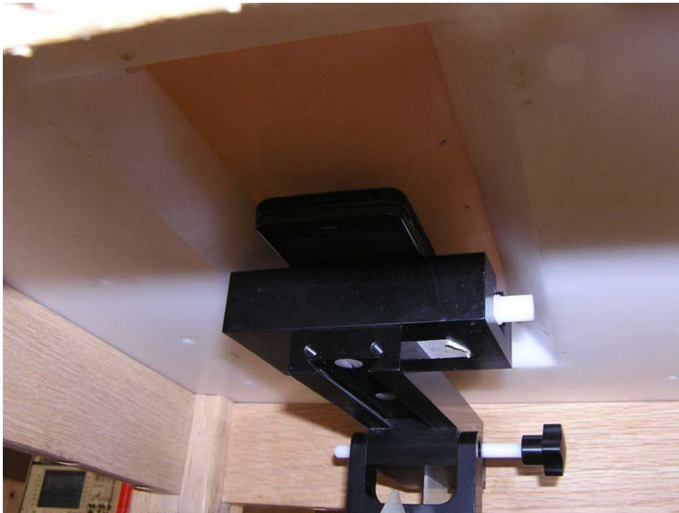
Figure 7: Mobile Hotspot Position at 10mm away from phantom (back of phone)
