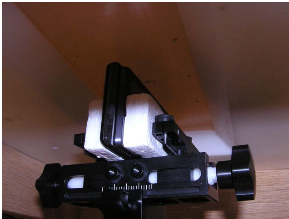
Figure 8: Mobile Hotspot Position at 10mm away from phantom Long edge of phone (right or left)
