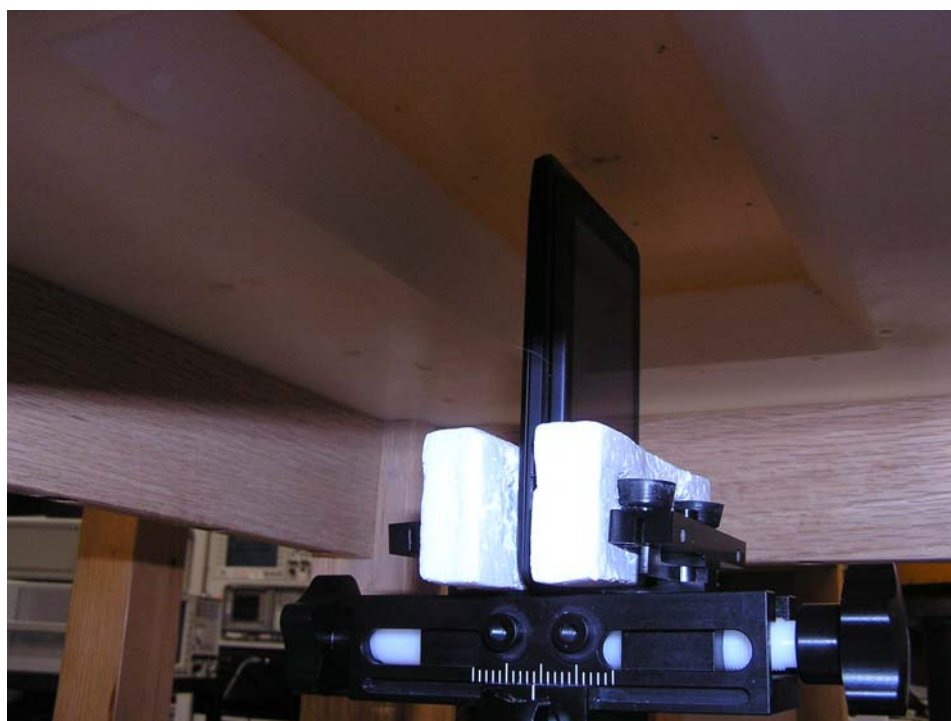
Figure 9: Mobile Hotspot Position at 10mm away from phantom Short edge of phone (top or bottom)
