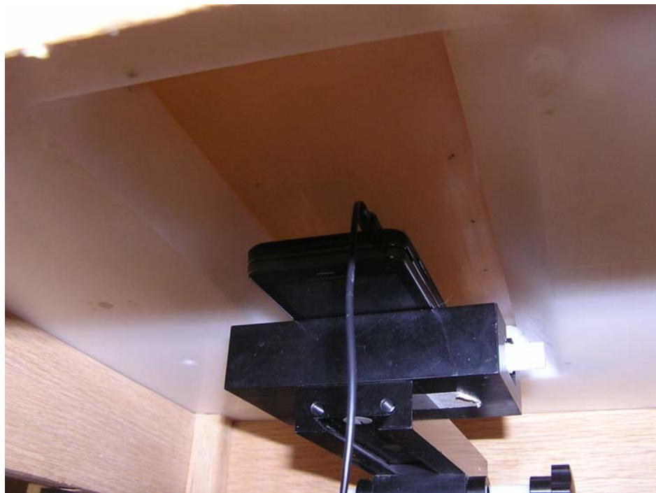
Figure 6: Body Position at 25mm away from phantom (back of phone)
