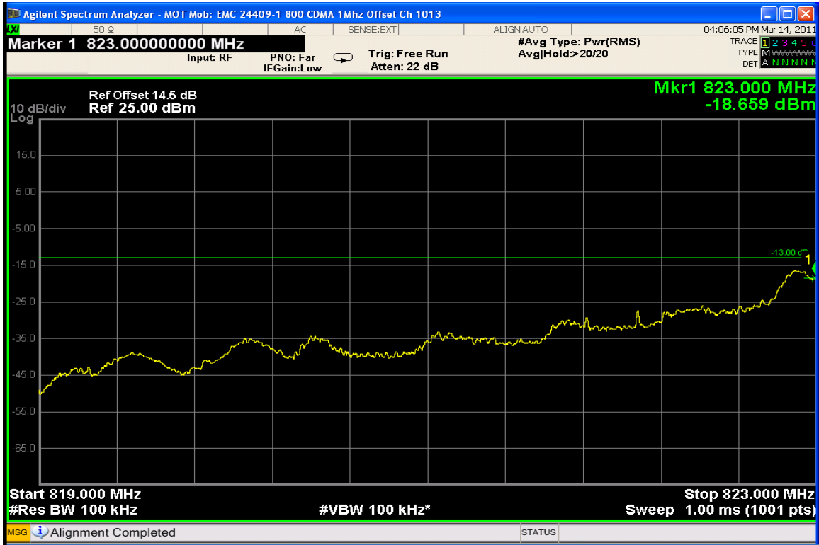
CDMA 800 Conducted Spurious Emissions (Lower adjacent 1 MHz band)
