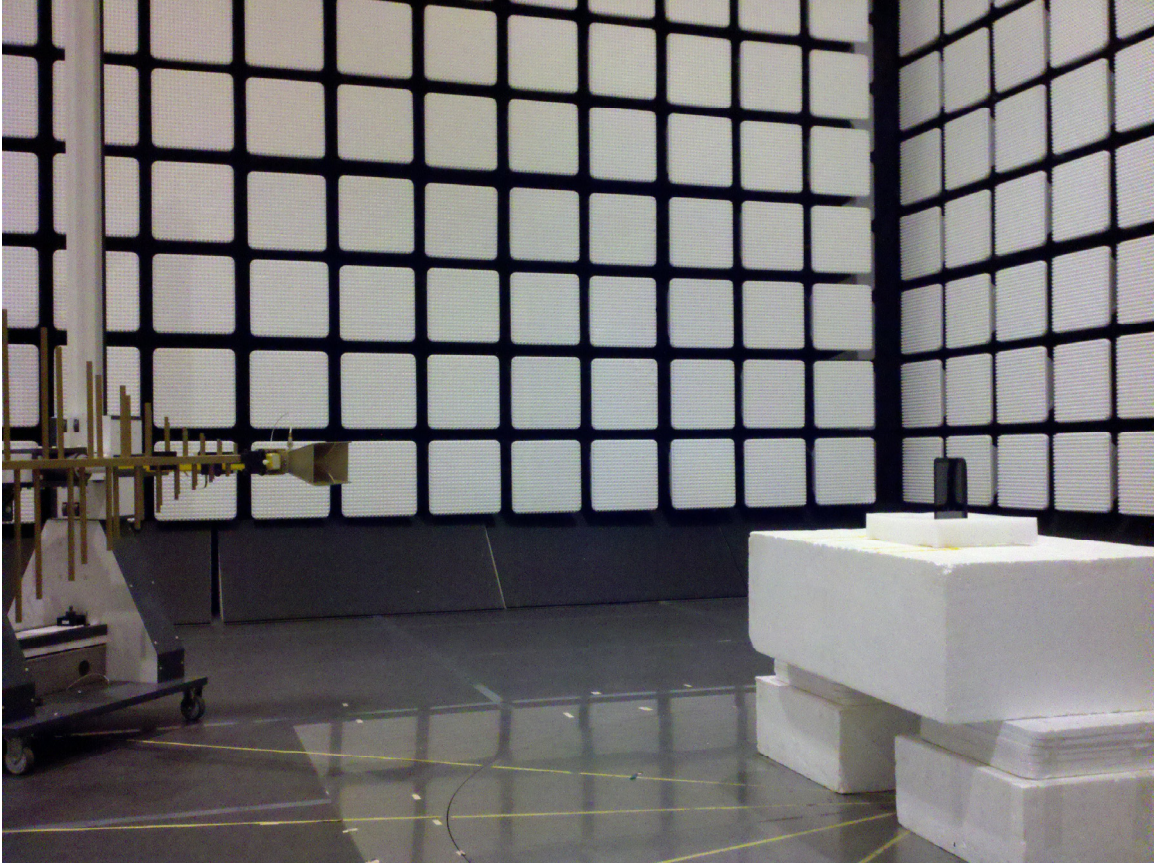
Radiated Emissions for BT & WLAN - BJ
