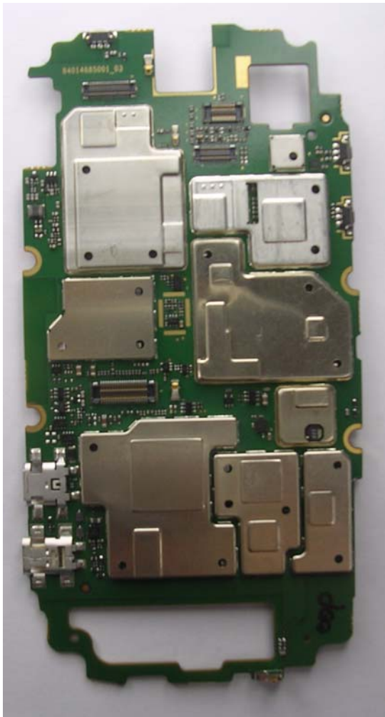
Front side of the main PCB with Shields
