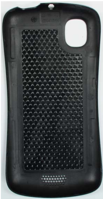
Battery door Inside
