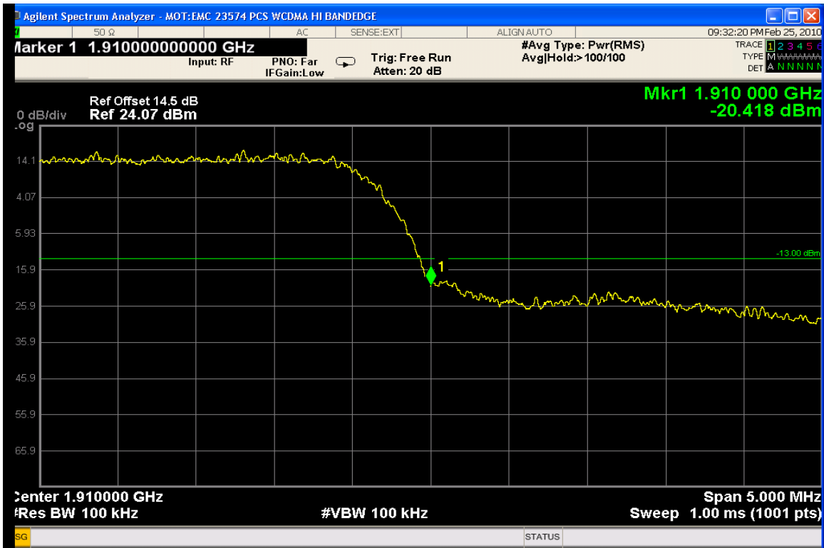
WCDMA 1900 – Upper Band Edge – Channel 9538 (1907.60 MHz)
