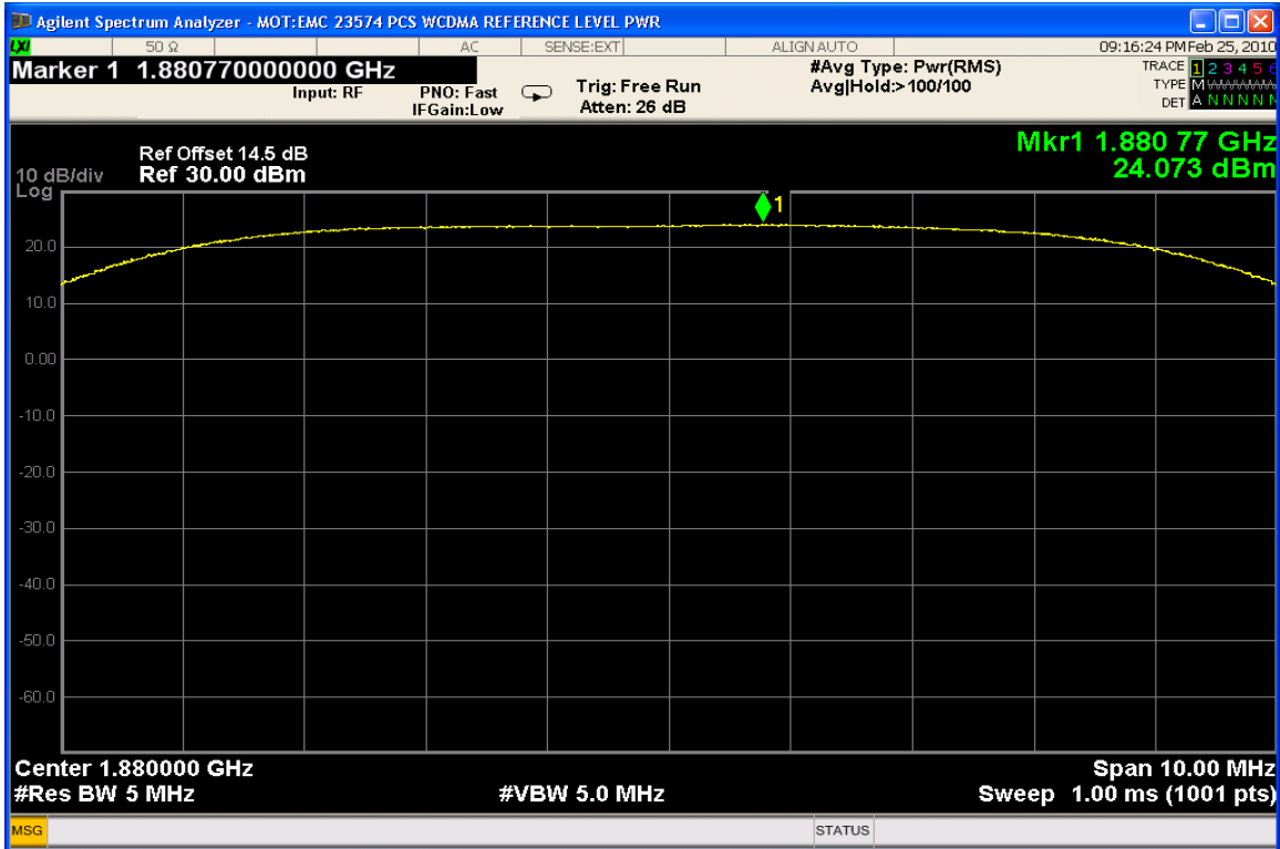
WCDMA 1900 – Reference Level Plot – Channel 9400 (1880.00 MHz)
