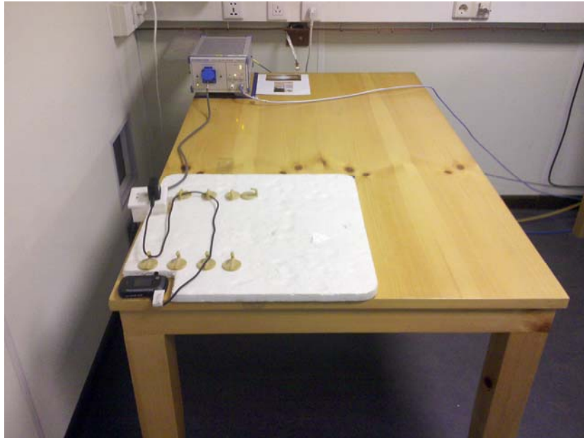
AC Line Conduct Emission
