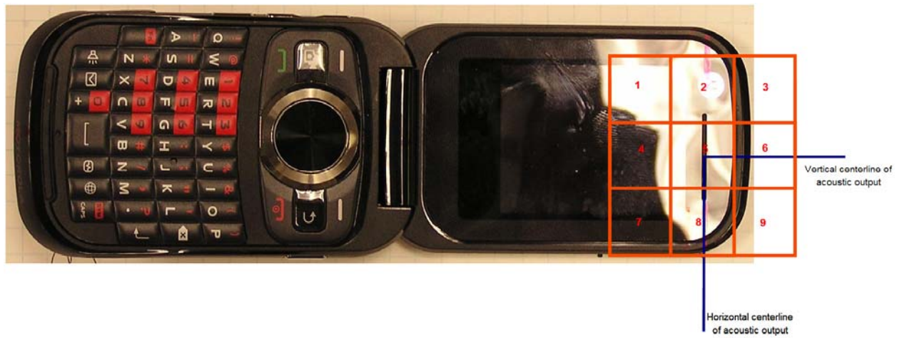
Figure 2. Phone Front - Orientation and Measurement Plane for RF Emissions Testing
