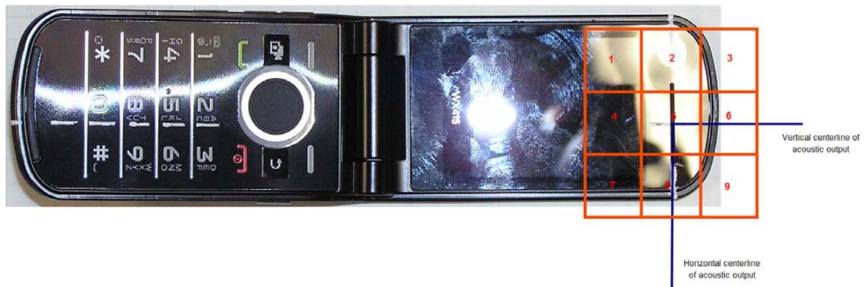
Figure 2. Phone Front - Orientation and Measurement Plane for RF Emissions Testing
