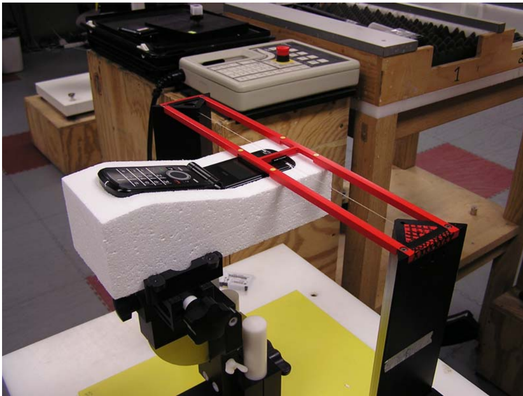
Figure 4. Positioning and Measurement for RF Emissions
