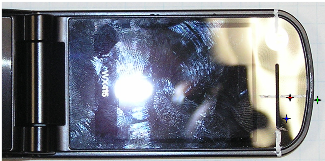
Figure 3. Phone Front - Location of Measured Points for Telecoil Emissions Testing
