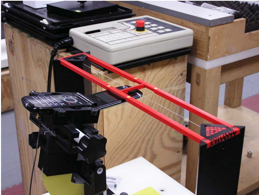
Figure 5. Positioning and Measurement for Telecoil Emissions
