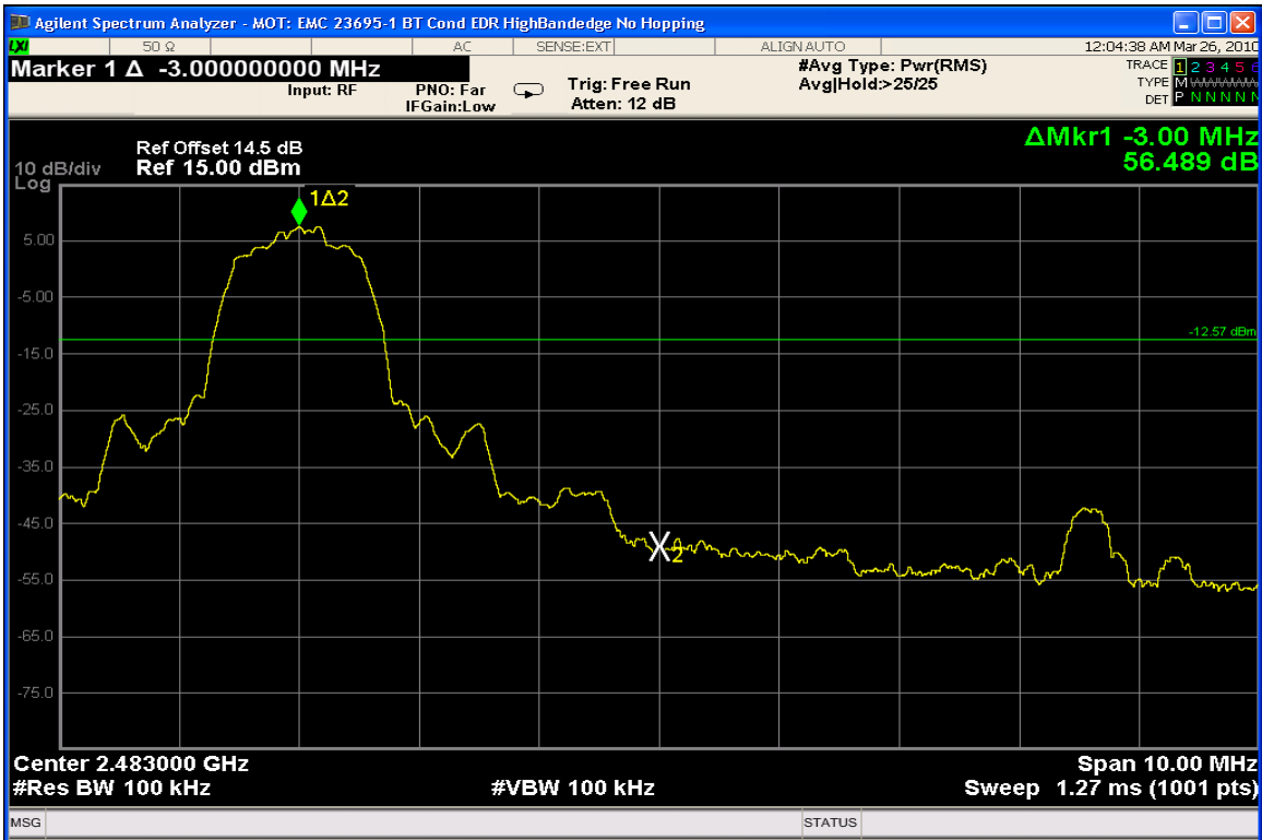
High Band edge with Hopping Disabled and EDR Enabled
