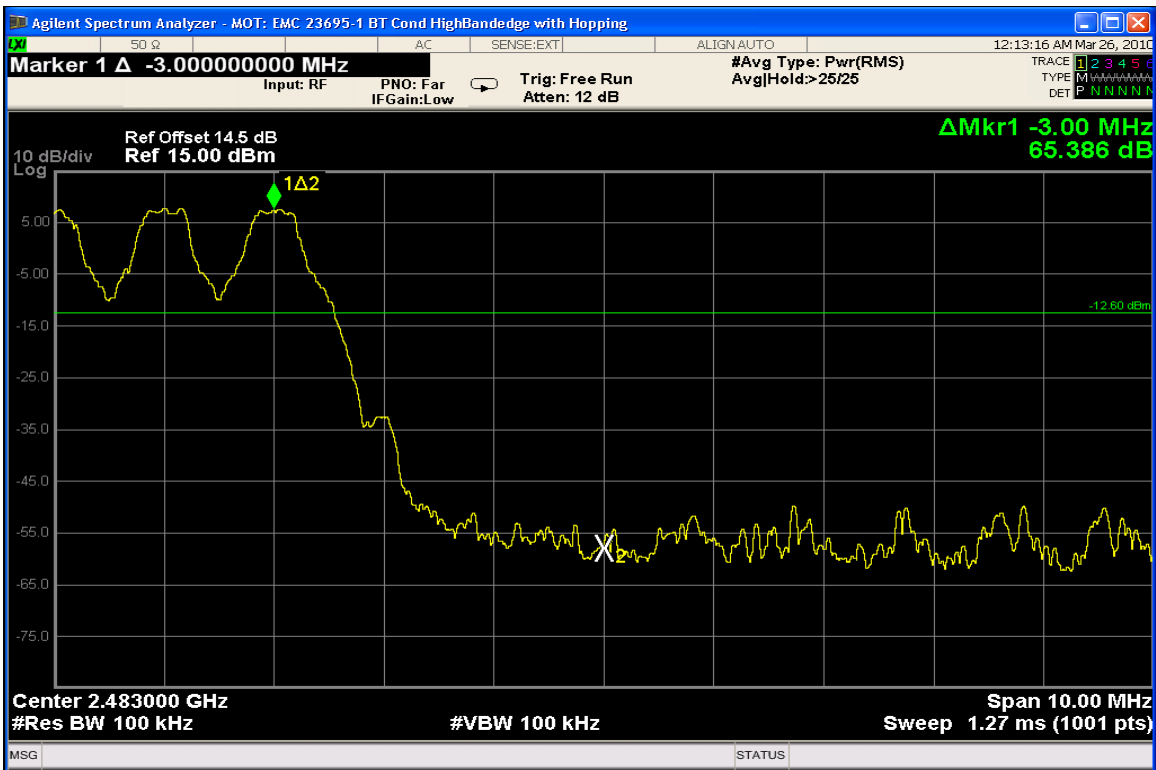
High Band edge with Hopping Enabled and EDR Disabled
