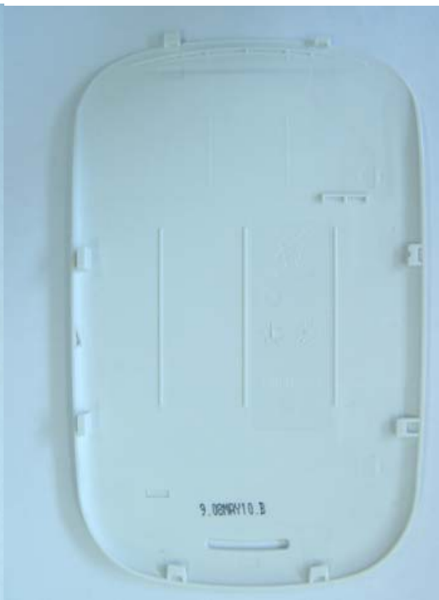
Battery door Inside
