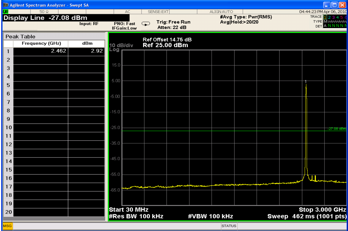
Conducted Spurious Emissions 30-3000 MHz (High Channel)
