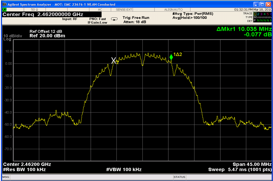
6 dB Bandwidth Channel 11 @ 1 Mbps
