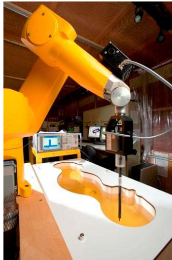
Figure 3-2 DASY4 SAR Measurement System
