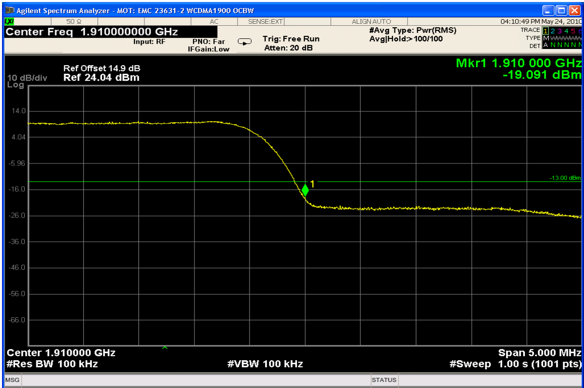
WCDMA 1900 – Upper Band Edge – Channel 9538 (1907.60 MHz)
