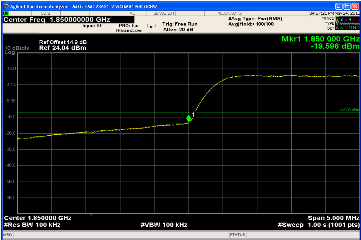
WCDMA 1900 – Lower Band Edge – Channel 9262 (1852.40 MHz)
