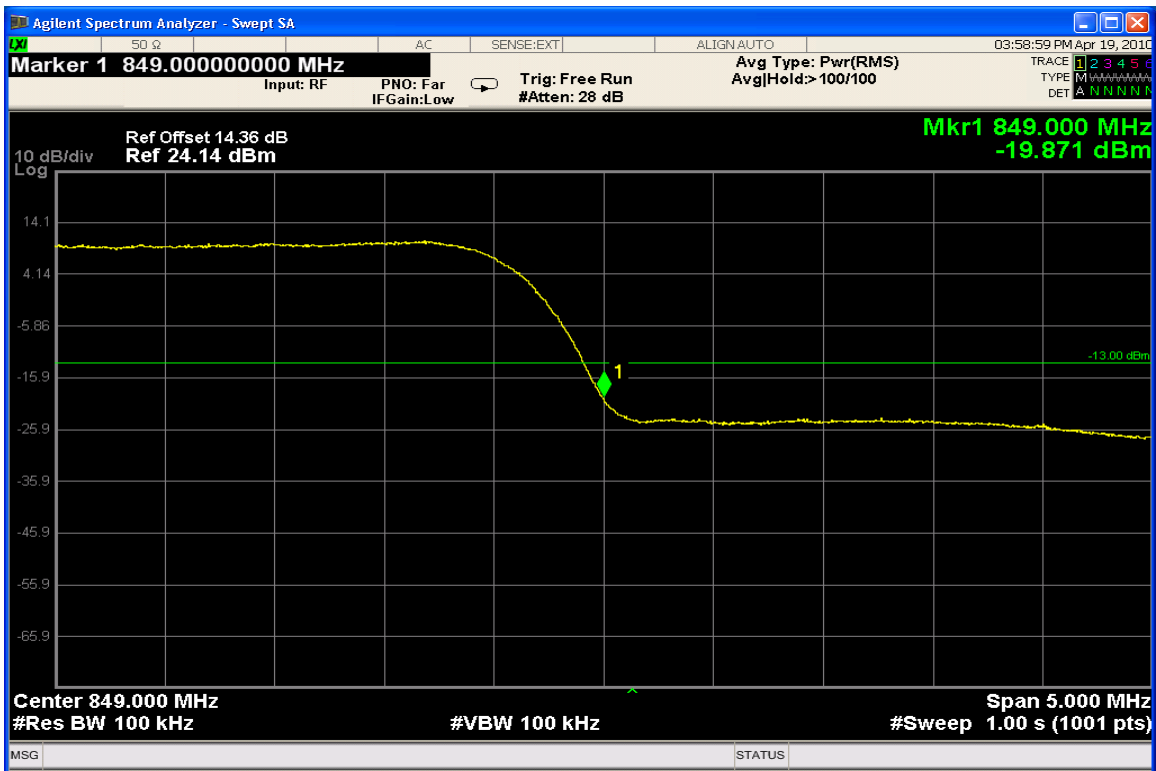
WCDMA 850 – Upper Band Edge – Channel 4233 (846.60 MHz)
