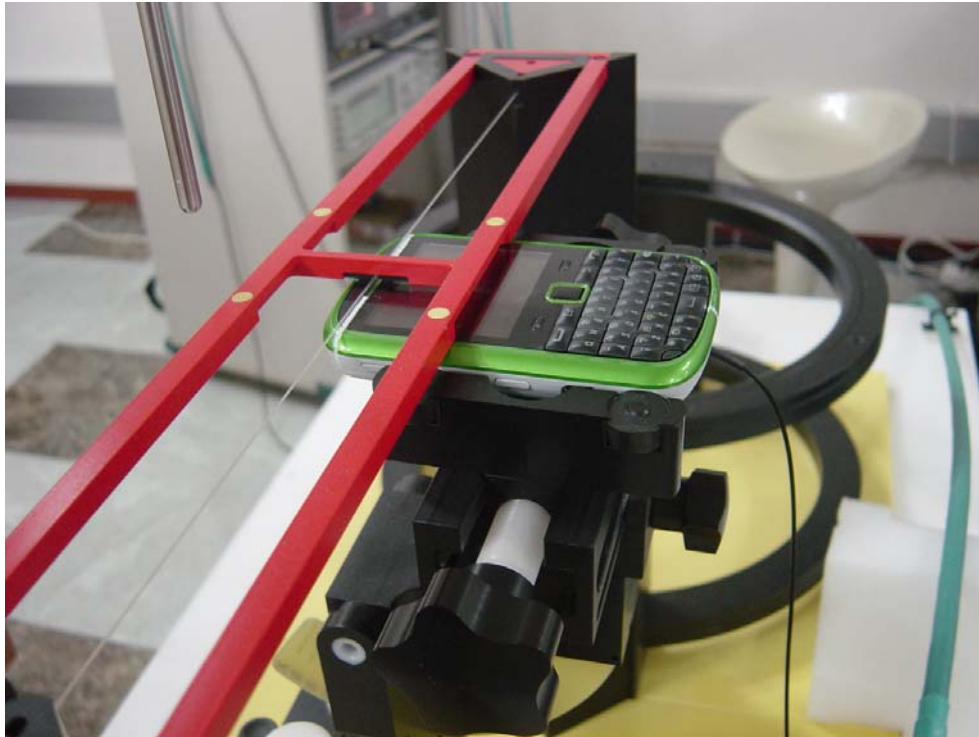
Figure 7. Positioning and Measurement for T-coil
