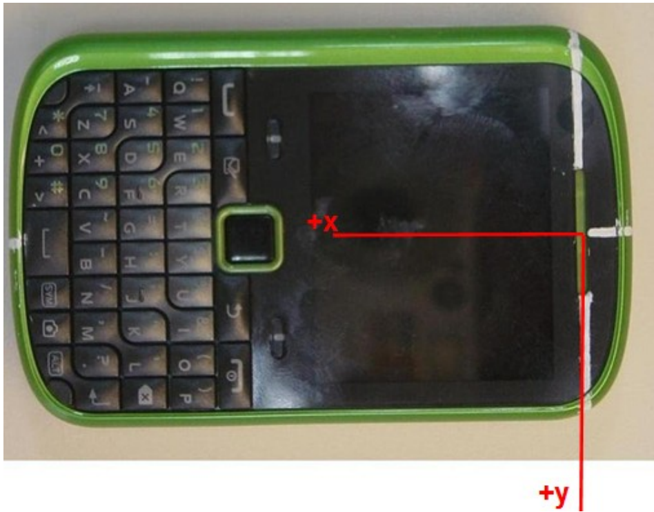
Figure 5. Coordinate Axis for T-coil Measurements
