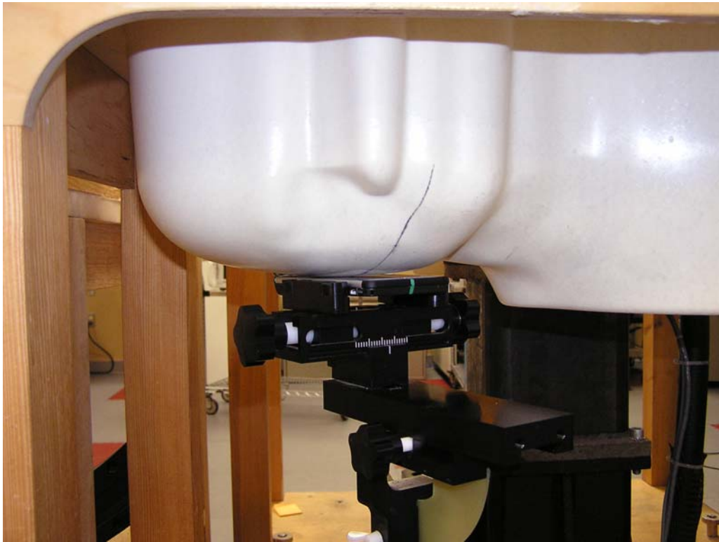
Figure 2: Cheek Position, Front of SAM Phantom
