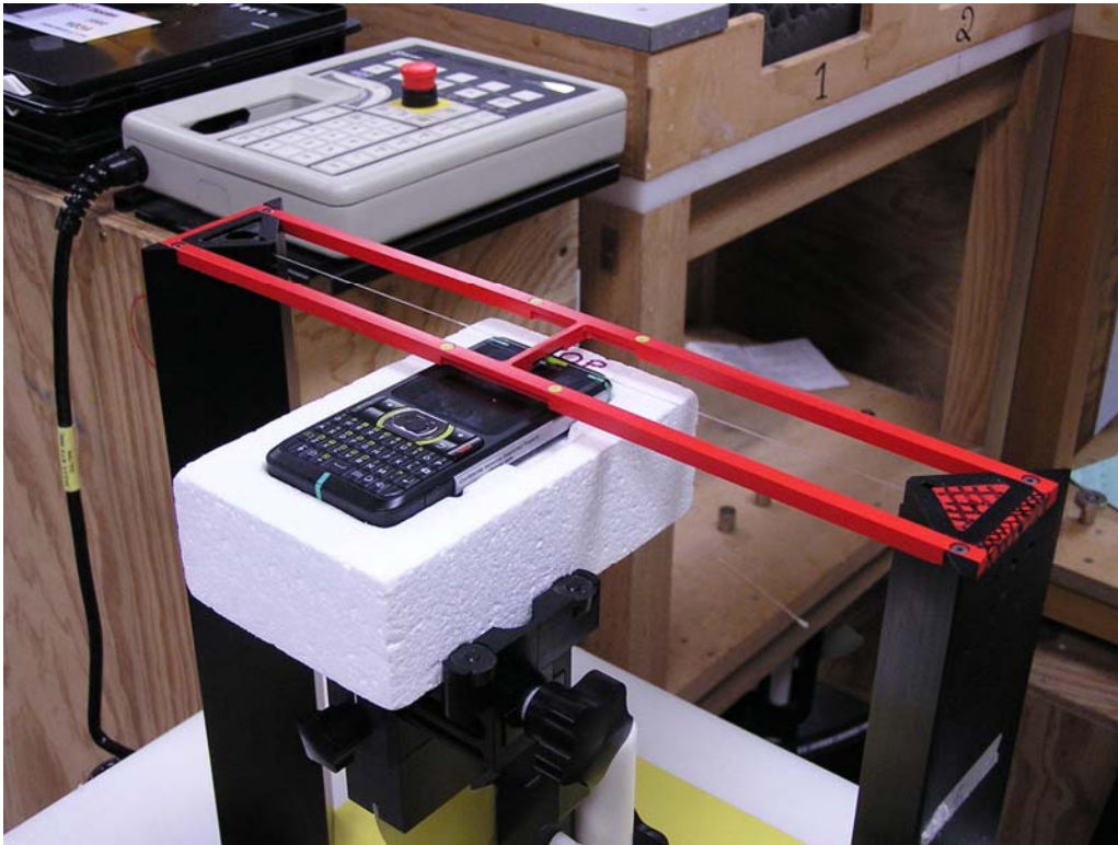
Figure 3. Positioning and Measurement for RF Emissions
