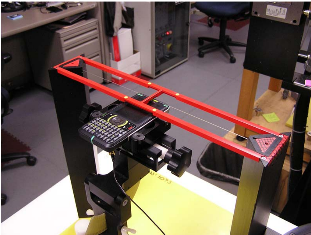
Figure 4. Positioning and Measurement for ABM (Telecoil) Emissions
