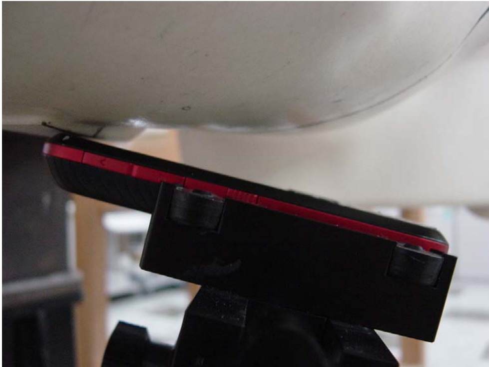
Figure 4: Phone Against the Head Phantom (15° Tilt)
