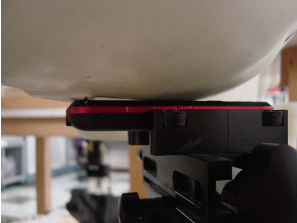
Figure 3: Phone Against the Head Phantom (Cheek Touch)
