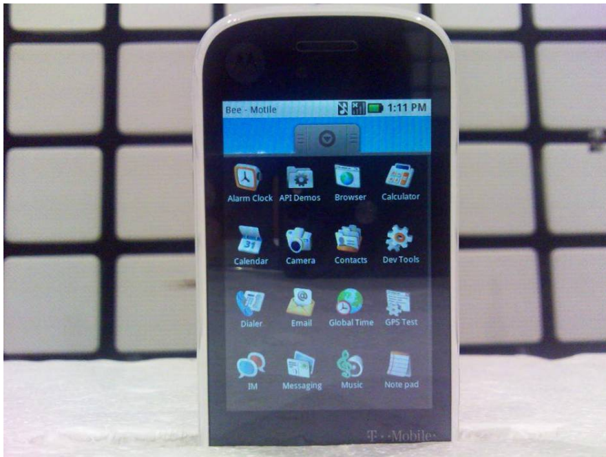
23305-1, IHDT56KV2 placed in test position Z – slider closed
