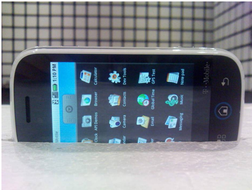
23305-1, IHDT56KV2 placed in test position Y – slider closed
