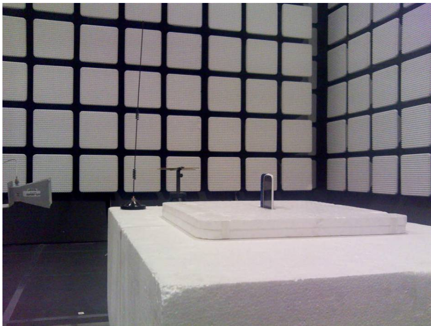
23305-1, IHDT56KV2 setup in semi-anechoic chamber – right view (18 GHz – 26.5 GHz)
