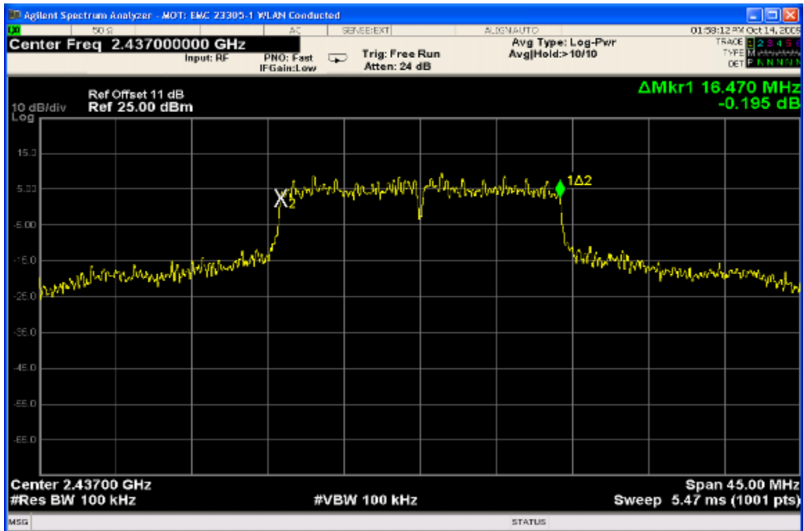
6dB Bandwidth Channel 6 @ 54 Mbps
