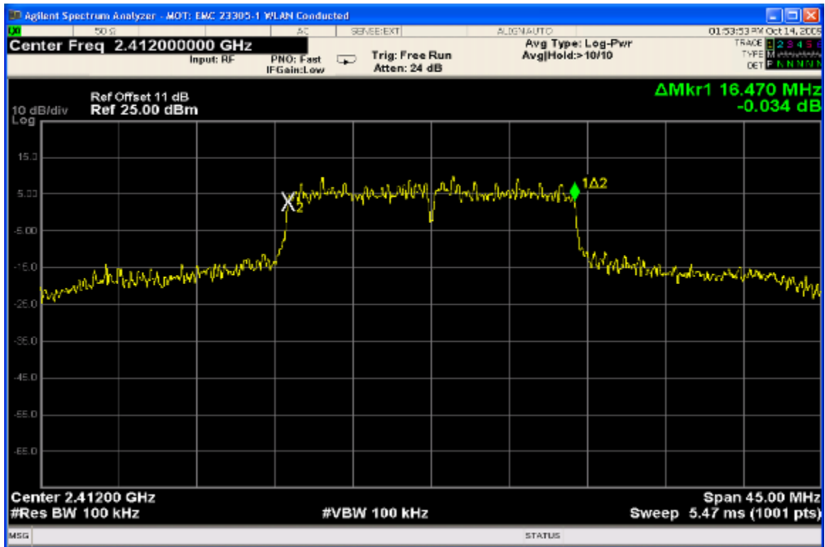
6dB Bandwidth Channel 1 @ 54 Mbps
