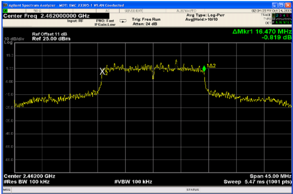
6dB Bandwidth Channel 11 @ 54 Mbps
