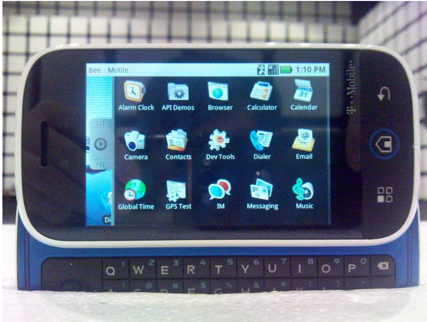
23072-1, IHDT56KV1 placed in test position Y – slider open
