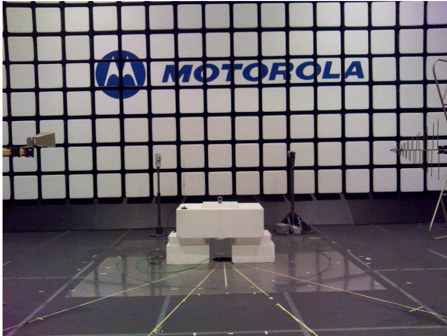
23072-1, IHDT56KV1 setup in semi-anechoic chamber – front view (30 MHz – 18 GHz)
