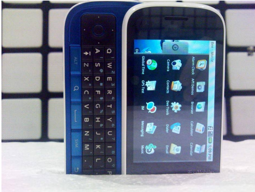
23072-1, IHDT56KV1 placed in test position Z – slider open
