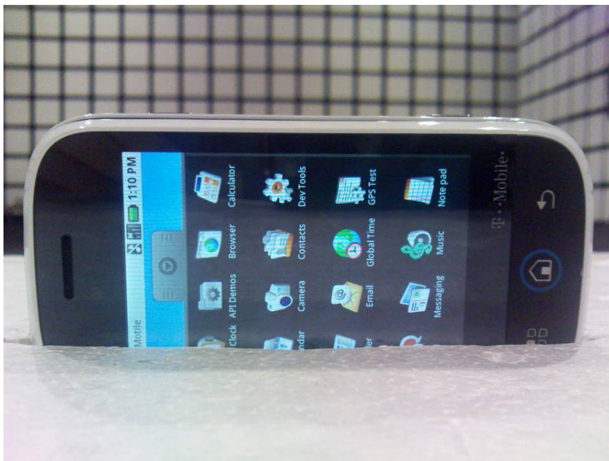
23072-1, IHDT56KV1 placed in test position Y – slider closed
