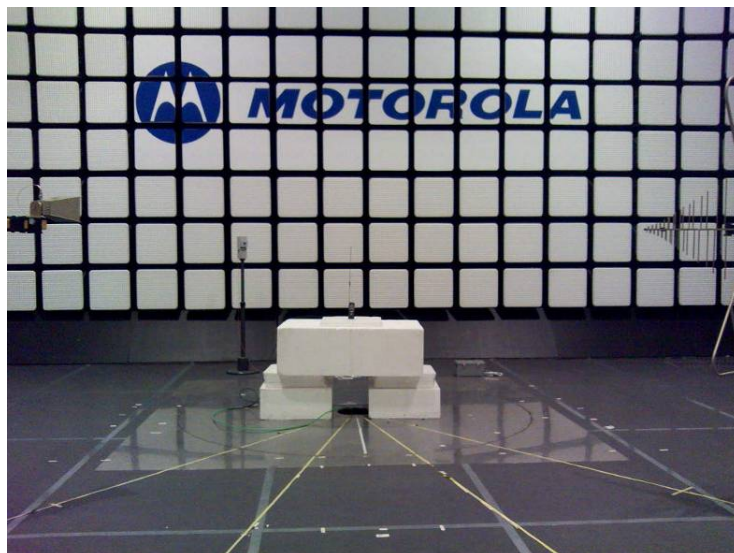
23145-1, IHDT56KS1 setup in semi-anechoic chamber – front view (30 MHz – 18 GHz)
