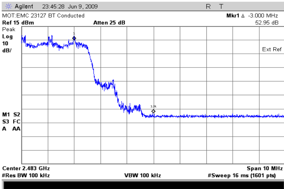
High Band Edge with Hopping Enabled (EDR MODE)
