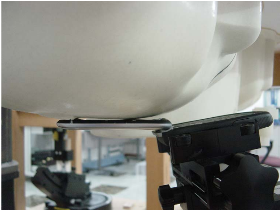
Figure 5: Phone Against the Head Phantom (Cheek Touch)
