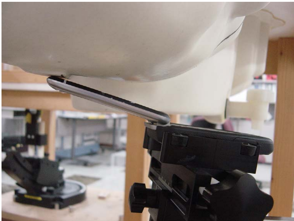
Figure 6: Phone Against the Head Phantom (15° Tilt)
