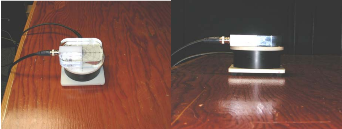
Figure 6-1 – Probe coil being calibrated with TMFS
