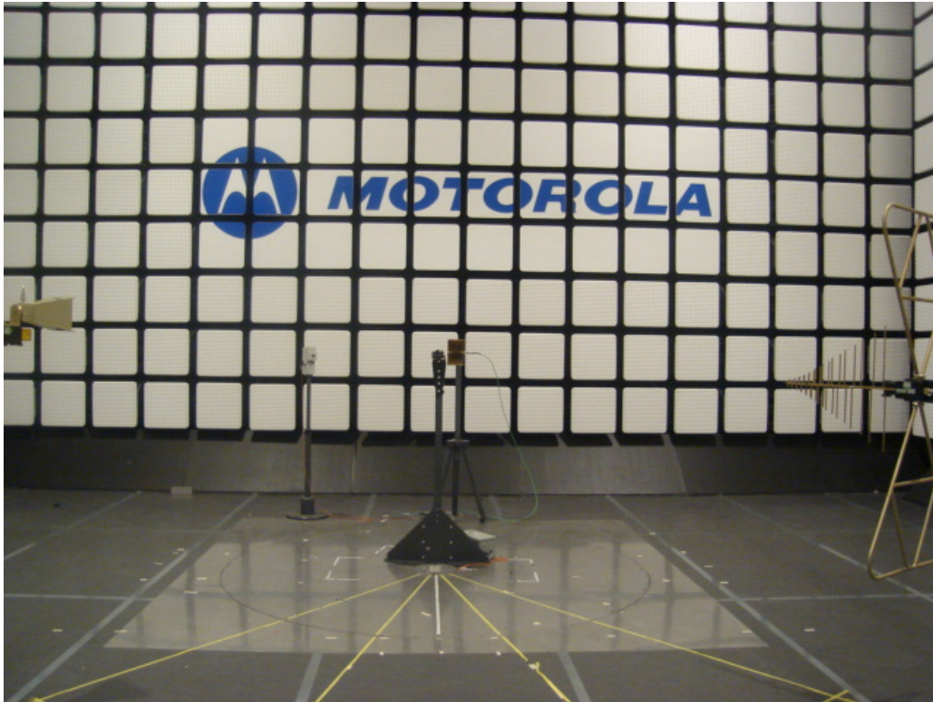
22719-1, IHDT6KP3 setup in semi-anechoic chamber – front view (30 MHz – 18 GHz)
